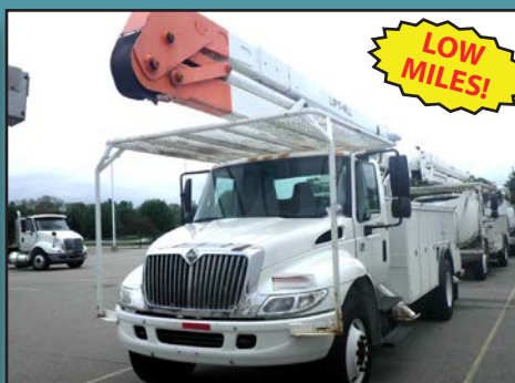
2007 INTERNATIONAL 4300 Bucket Truck IHC DT466/245hp, Allison automatic transmission, 12,000# front axle, 21,000# rear axle, spring suspension, 15' utility bed, 55' Lift All 2 man bucket, 4 outriggers, 188" w.b. ONLY 55k Miles!!!
