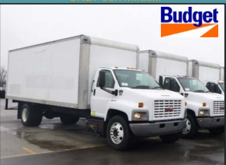
Group of 2006 GMC C7500 Box Trucks Caterpillar C-7/190hp, automatic transmission, spring suspension, 24' box, roll up rear door 260" w.b.
